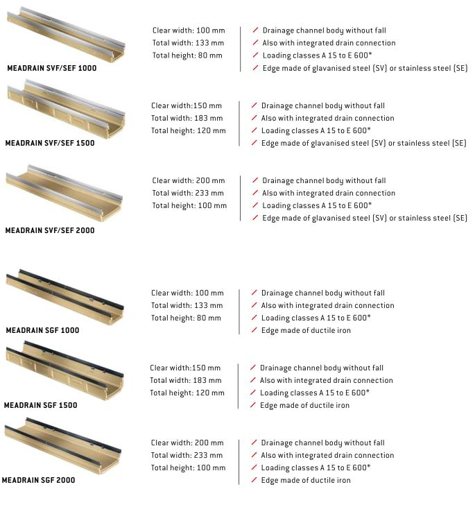
\* From loading class D 400 not suitable for cross drainage of high speed roads and motorways.
